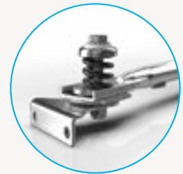
Rosco's heavy duty detent system has the greatest holding power in the industry with the most robust spring, lock and wear plates, and stainless steel hardware. This design keeps the mirror arm where the driver needs it under highway wind loads, while also allowing for bi-directional impact breakaway and folding (during parking).
