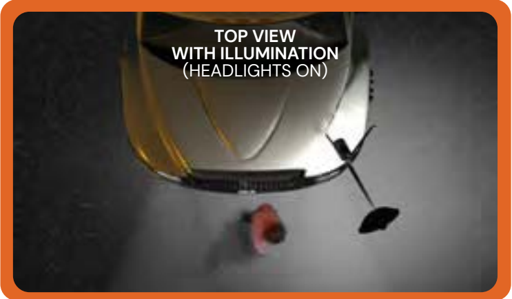
WITH ILLUMINATION With the new LED under mounted lights, objects and pedestrians in front of the bus are clearly visible to the driver.
