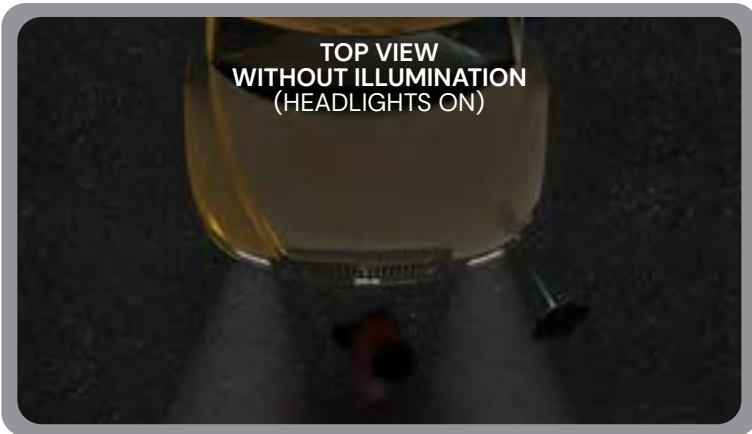
NO ILLUMINATION In low light conditions, the reflection in any mirror is difficult to see. An object or pedestrians in front of the bus may be almost invisible.
