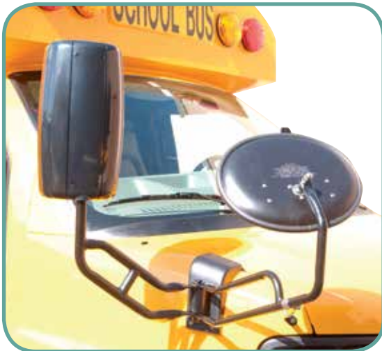
Ford E-Z Bracket® Installation with Model 815U AccuStyle® and Hawk-Eye® Cross View Combo Assembly
