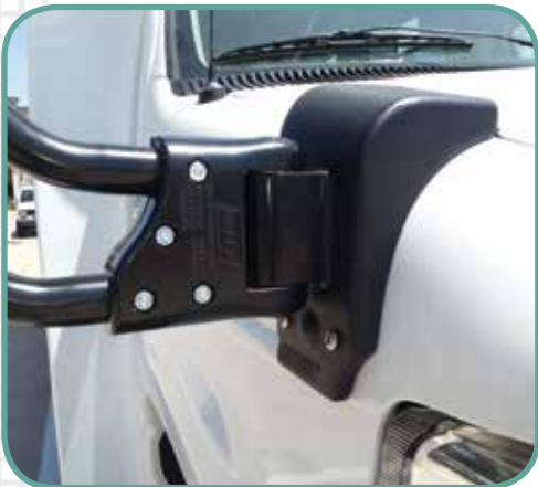
Fender Mount Rearview Mirror Assembly with Spring-Break® Detent (Non Combination Assembly)
