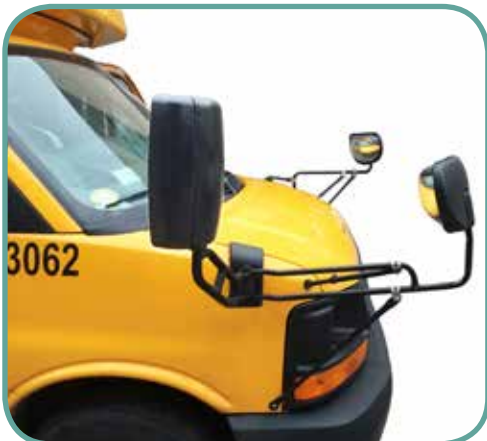
GM E-Z Bracket® with Model 815 AccuStyle® and Eye-Max® LP Cross View Combo Assembly
